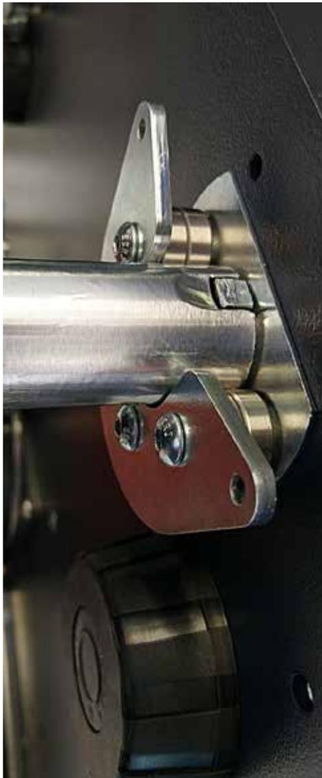
Drive via bolt-groove connection
